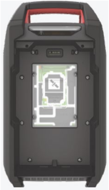
Figure 1-12: Satellite Connection Installed
