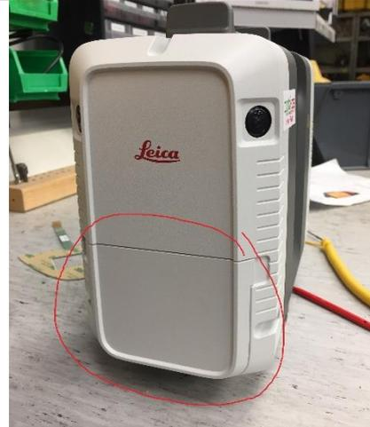
The serial number and identifying the scanner can be found on the area marked opposite.
