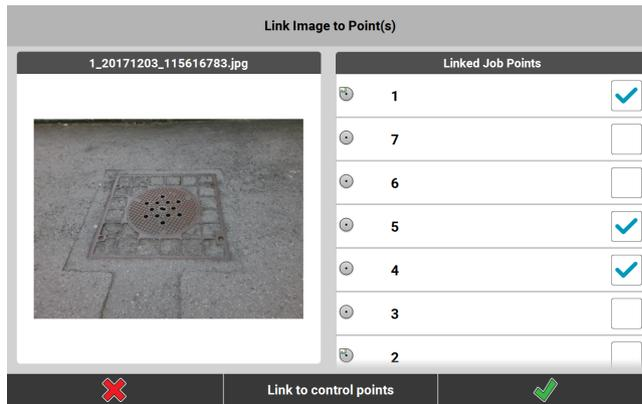
3. Activate the checkbox of a point to link it to the image.
