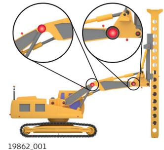
Point B2 is optional, but must be measured when the driller has dual boom.
