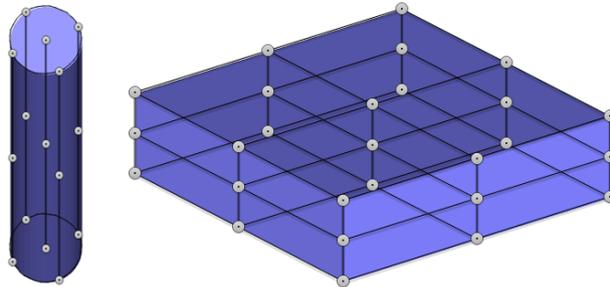
For cylindrical objects such as pipes or columns, the following points and lines are displayed to simplify the layout process:
