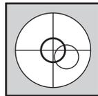
Before determining the instrument errors, the instrument has to be levelled using the electronic level. The tribrach, the tripod and the underground should be stable and secure from vibrations or other disturbances.
