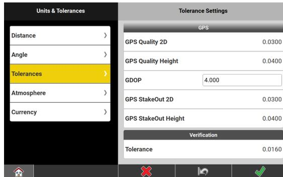
3. In the **Tolerance Settings** screen, define the **Tolerance** level. Select from three predefined tolerance sets:
