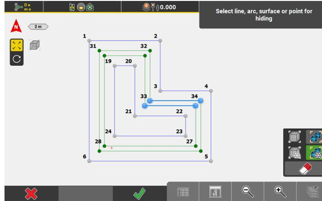
*As soon as an element is selected, a preview of the isolation mode is given: selected elements are highlighted in blue, elements of the same layer are highlighted in green. All remaining elements are displayed in their original colour.*
