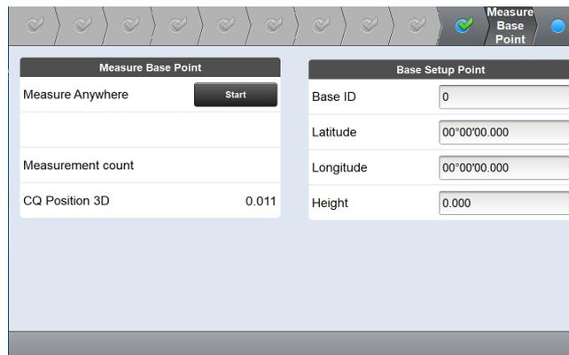
5. If the quality of the measurement is sufficient, tap **Stop** to store the measured base point.
