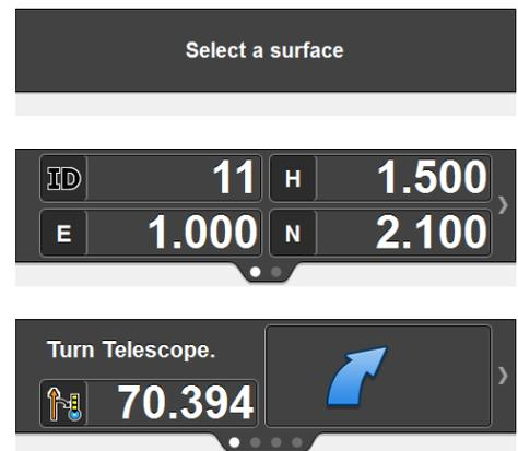
The white dots at the base of the Information bar indicate the total number of active pages, which can be scrolled through by tapping on the left hand side or right hand side of the Information bar.
