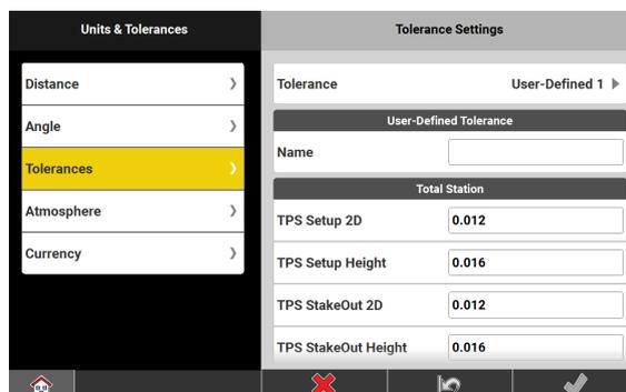
Adopted tolerance values differ according to the connected instrument, and the active application:
