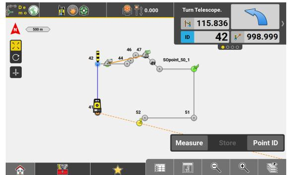
2. Configure the Measure bar to display **Point ID**, then tap **Point ID**. Tap on the **Point ID** tick box and tap
