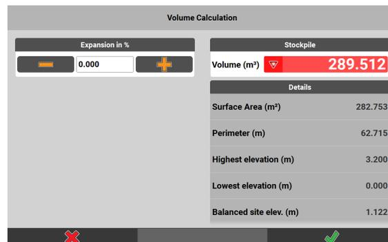
*The calculated volume of the selected surface along with measurement data is displayed.*
