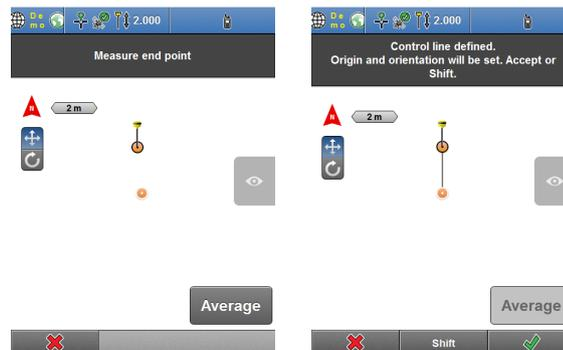
4. - To Shift the origin of the control line, press **Shift**.
