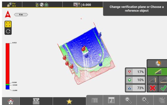
The heatmap shows the verification plane with the result overlaid. A quantity indicator shows the percentage of the points in tolerance and out of tolerance, above and below the verification plane.
