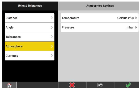
3. In the **Atmosphere Settings** screen, set the units for **Temperature** and **Pressure**.
