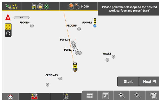
4. *The instrument starts measuring and turns automatically to the desired coordinates (X, Y) on the existing ceiling or floor.*
