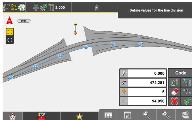
4. Use the toolbar to define the values for line division and if necessary, the values for offsetting the segment points. The map view is updated accordingly to show a preview of the points to be created.
