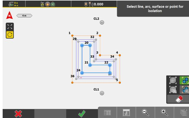
*As soon as an element is selected, a preview of the isolation mode is given: selected elements are highlighted in blue, elements of the same layer are highlighted in orange. All elements to be hidden are displayed in their original colour.*
