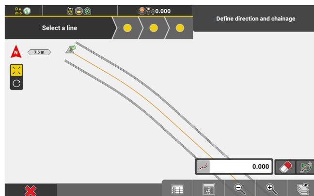
Select a line to be used as road line. If necessary, define direction and chainage of the road line in the toolbar.
