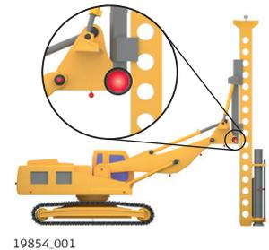
Point TD located at the bottom of the tower.
