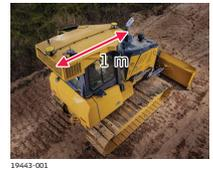
6. Mount a prism or a tape at the centre of the blade to measure the ARP points (arm rotation point). Make sure you measure always the same spot with 0 m prism height.
