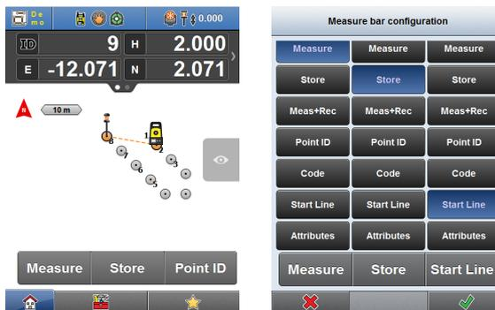
2. Press **Start Line**. Measure and store points. A line is drawn between the points.
