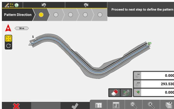
Select two points, a line or a polyline to define the forward direction of the pattern.
