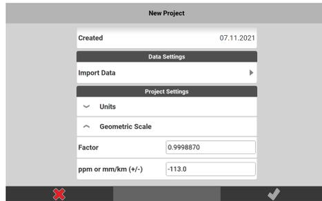
The geometric scale factor can only be set when creating a project. Input the desired value under **Geometric Scale**.
