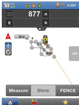
*The code key in the Measure bar displays the selected code. The selected code is assigned to any points that are stored.*
