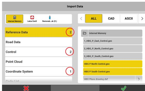
*For each data type, the software counts the number of selected files and displays it to the right of the data type name. Collapsed folders that contain selected files are marked with an orange dot.*
