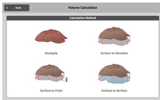
Select **Surface to Elevation** in the Calculation Method screen.
