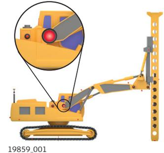
Points B and B2 located at the boom and stick joints.
