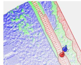
The software creates extrema points for out-of-tolerance areas, and contour lines to delimit the areas within and outside the tolerance. Contour lines for areas above the tolerance are coloured red, contour lines for areas below the tolerance are coloured blue.
