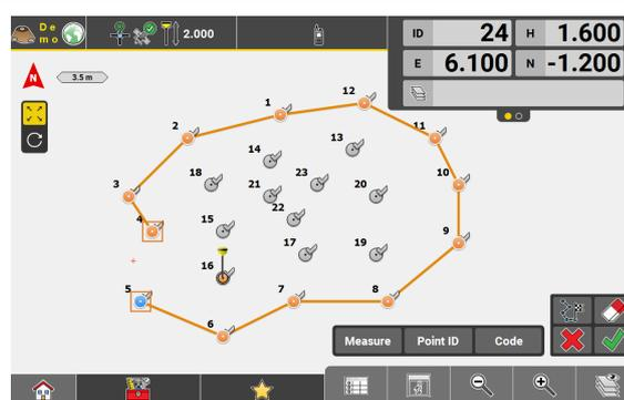
The boundary is displayed in orange colour. Open boundary points are highlighted by an orange box:
