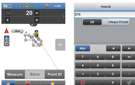
☞ To recall this function automatically for every measured/stored point, tap the **Always Prompt** checkbox.
