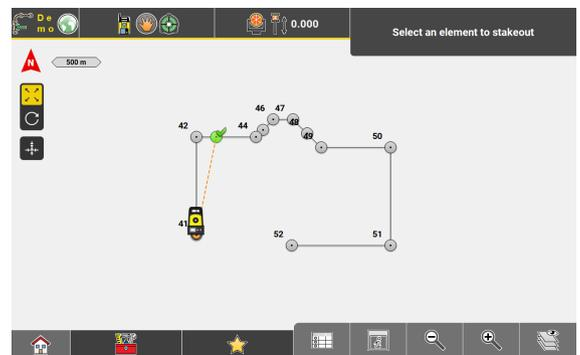
☞ In 5" or 7" display mode, with Multiview active, use **Stakeout Point List** to get the points to be staked displayed. It is possible to select the points for staking out in the list.
