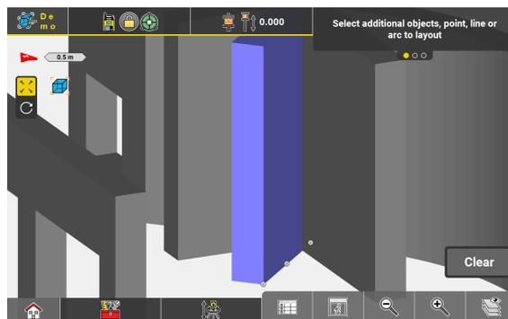
*When the IFC object is selected again, only the user-defined wireframe points are visible.*
