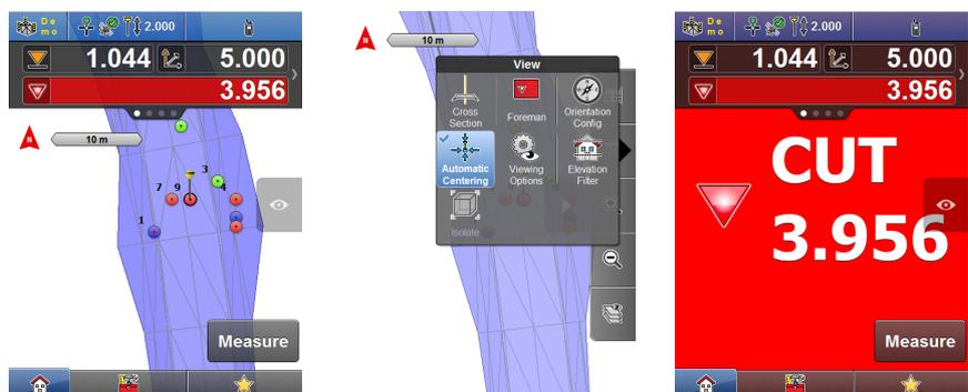
☞ The Cut/Fill tolerance level can be selected in **Tolerances**, which is found in **Units**
