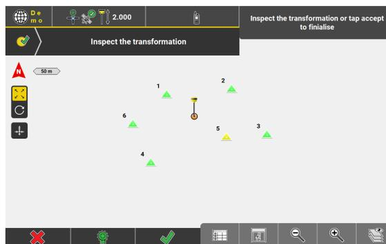
The Map screen is then displayed showing the points that shall be used for the transformation.
