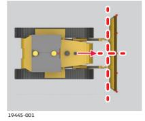
5. Mount the GNSS antennas as close as possible to the centre axis of the machine and at least 1 m apart from each other.
