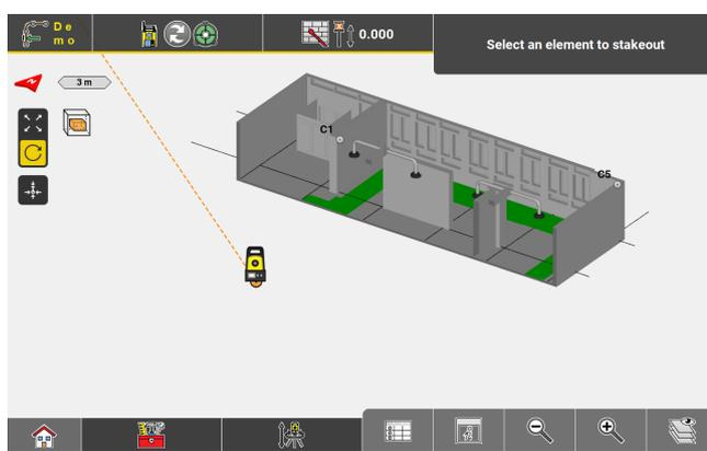
Elements outside the defined limit box disappear from the map view. While the Limit Box is active, the Limit Box icon is displayed in the top left corner of the map view.
