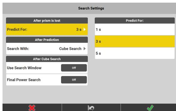
In the **Search Settings** screen define the behaviour of the Total Station after a prism loss.
