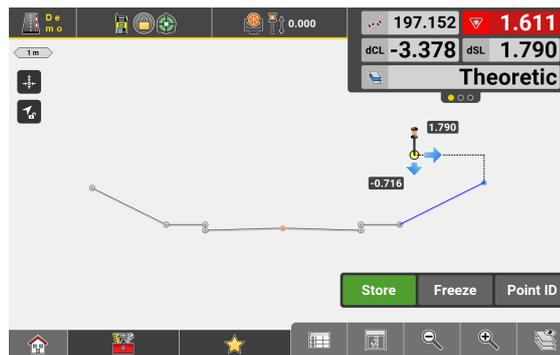
The view mode changes into cross-section. The target is shown against the current cross-section of the selected road model.
