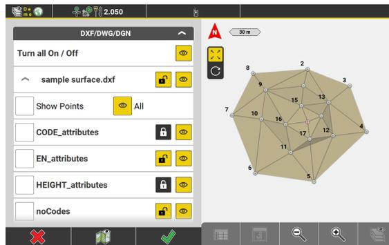
When the button is "on"
