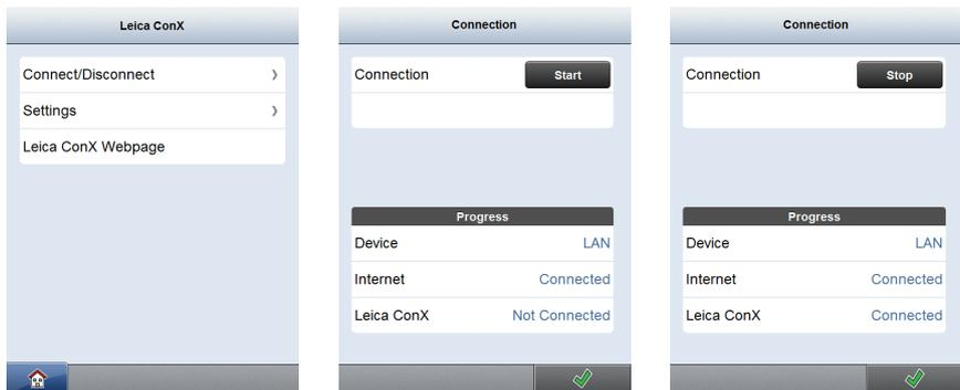
☞ The device is connected to the Leica ConX web page now and ready for **View**, **Sync** and **Track**.
