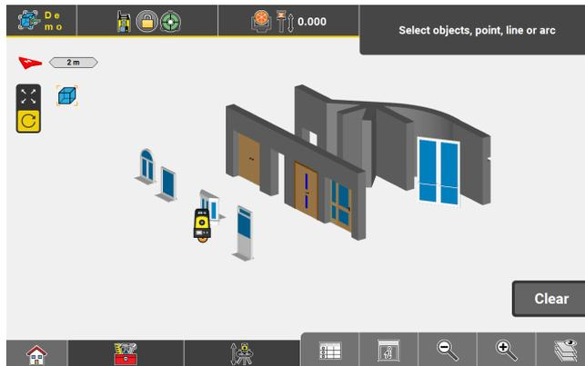
To indicate that isolation mode is active, the **Isolate** icon is displayed in the top left corner of the map view. The icon disappears when all objects are visible in the map view.
