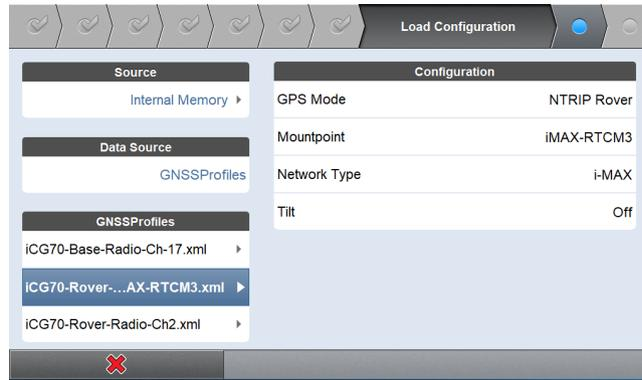
3. For a radio rover profile, define the internal radio settings. For a network rover profile, define the network and mountpoint settings.
