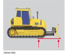
4. Make sure that the blade is perpendicular to the machine direction.
