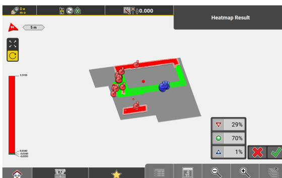
The heatmap shows the reference object with the result overlaid. A percentage indicator shows the percentage of the points in tolerance and out of tolerance, above and below the reference data.
