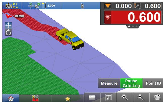
You can pause grid logging at any time. Tap **Pause Grid Log**. To resume grid logging, tap **Start Grid Log** again.
