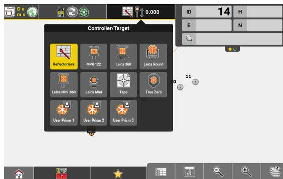
3. Select the prism type you want to use by tapping the relevant symbol, either from the default or the user-defined ones, for example **Leica 360**.
