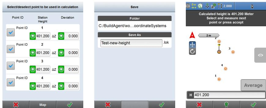
When more than one point has been measured to define the local reference height, a **best fit** solution will be applied and used as the height difference. This means that the local reference height is balanced from the measured heights and the height difference equals the height of the newly measured point minus the local balanced reference height.
