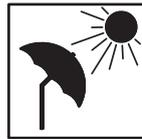
The instrument should be protected from direct sunlight to avoid thermal warming. It is also recommended to avoid strong heat shimmer and air turbulence. The best conditions are early in the morning or with overcast sky.
