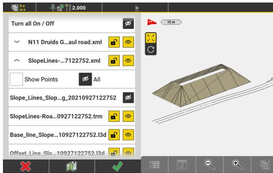
Surface, baselines and slope lines are stored on separate layers.
