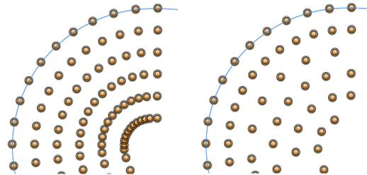
Define the maximum hole spacing to add extra holes. The added holes are shown in purple colour.
