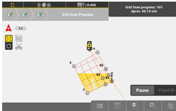
The info panel displays the progress and the estimated remaining time for scanning.
