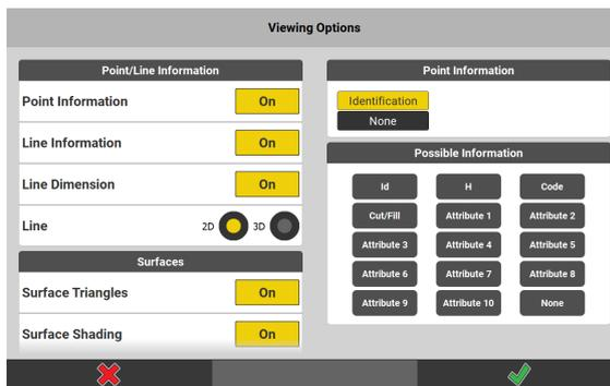
2D shows the horizontal line length as entered for distance. 3D shows the slope distance.
