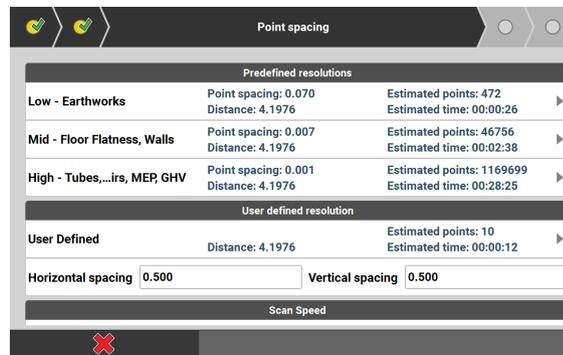
*The point spacing defines the resolution of the scan data. Depending on the selected point spacing, the software calculates the estimated number of scan points and the estimated scanning time.*
