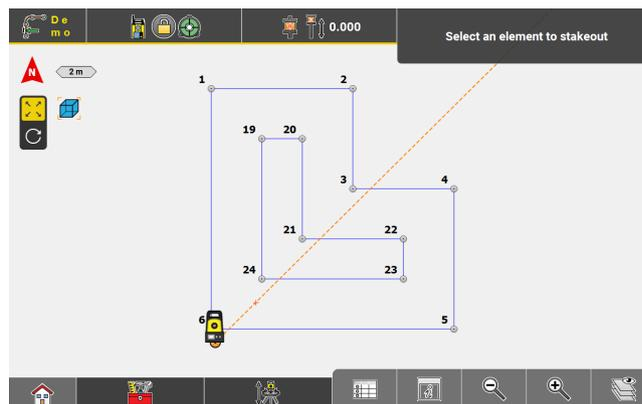
*To indicate that isolation mode is active, the Isolate icon is displayed in the top left corner of the map view. The icon disappears when all elements are visible in the map view.*
