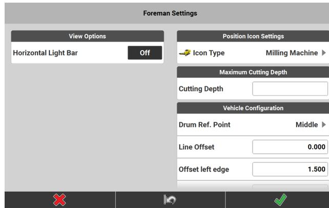
3. Enter the maximum cutting depth value of the milling machine. *Different milling machines have different maximum cutting depths. During milling, the software checks the height deviation between existing and design surface. If the height deviation is greater than the defined cutting depth, a warning is displayed in milling view. Areas where the cutting depth limit of the machine is exceeded need to be milled again.*
