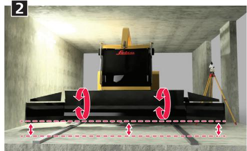
1. Fully extend the blade wings and level the blade.
