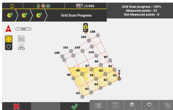
When the scanning process is finished, the info panel displays the scan result. All measured points are displayed on the map.
