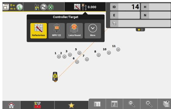
A subscreen displays the last three Prism types used, with the currently active Prism type being highlighted.
