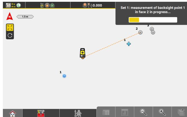
8. *As soon as the measurement process is finished, the residuals for each measured point are displayed.*
