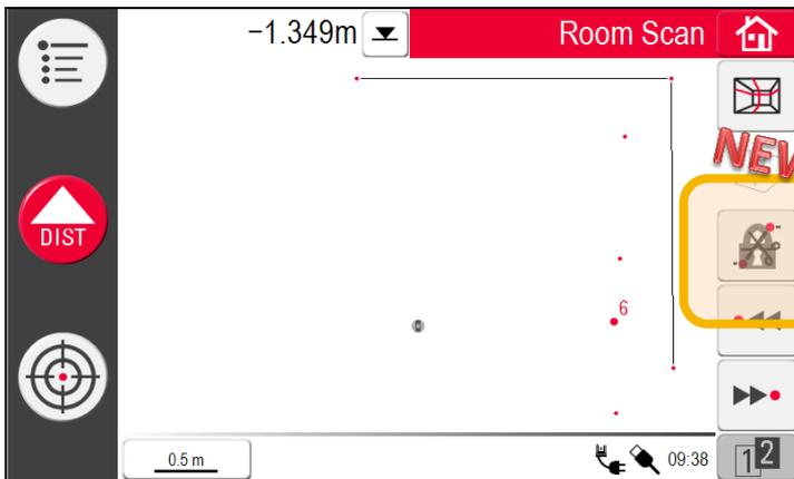
The Room Scan application's CUT LINE key is now lockable and enables to measure points without line connection. It is not necessary any more to delete the line afterwards.
