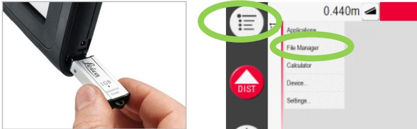
Plug the USB stick into the Control Unit.
