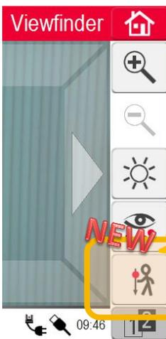
The Viewfinder's former Hidden Point tool was extended. New offset options enable to use different target plates or rods. Each offset measurement is documented in the CSV export file. Any rod of individual length can be used for indirect measurements.
