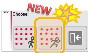
The Speed Scan offers a fast acquisition of the to be scanned surface. It runs several times faster than the normal Surface Scan and accuracy is the same – just with slight irregularities of the grid, which is acceptable for most use cases.
